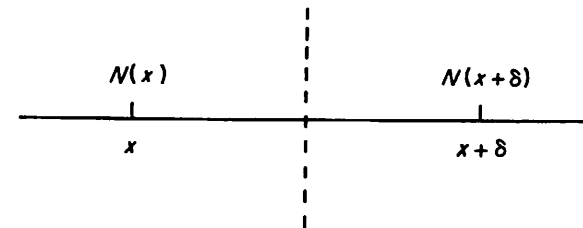
Fig. 2.1. At time t , there are N(x) particles at position x , N(x + \delta) particles at position x + \delta . At time t + \tau , half of each set will have stepped to the right and half to the left.
